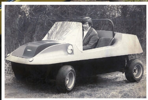
Barry with the Mini Bug-1 prototype, which featured a plywood bonnet, in 1969.
