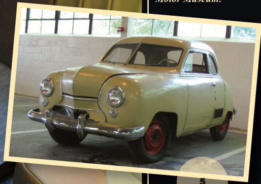
5 The rear-engine, front-wheel-drive Gregory sedan prototype in storage at Lane Motor Museum.
